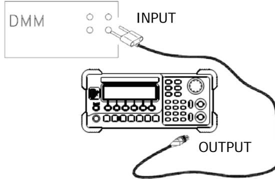
Figure 3-2 AC Amplitude Adjustment Connection
