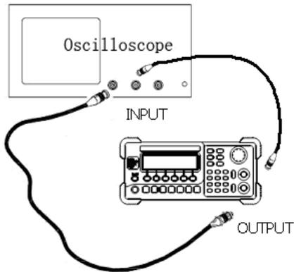
Figure 3-13 Phase Adjustment Connection
