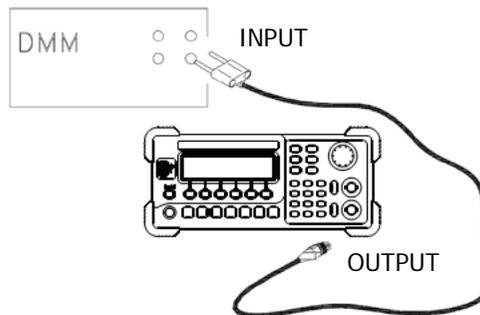
Figure 3-3 Offset DAC Connection
