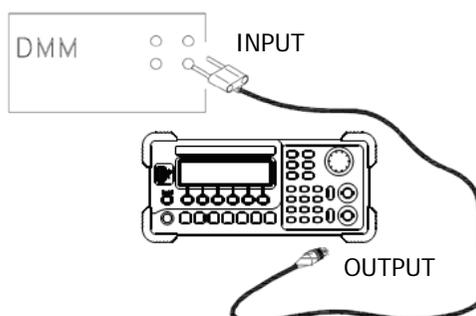
Figure 3-9 Low Frequency Flatness Adjustment Connection
