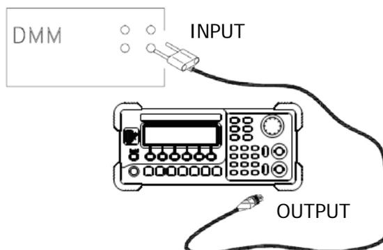
Figure 3-7 AC Amplitude Adjustment Connection
