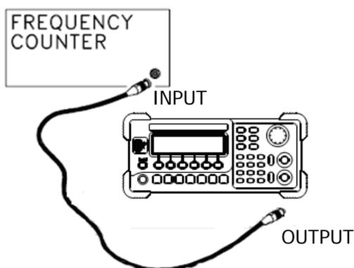
Figure 3-1 Frequency (Internal Timebase) Adjustment Connection
