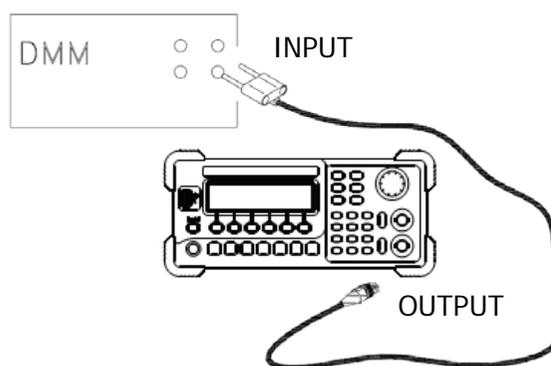
Figure 3-4 Low Frequency Flatness Adjustment Connection
