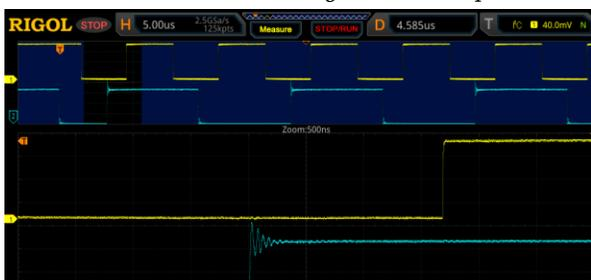
Figure 15: I2C clock and data min/max signal measurements using a RIGOL MSO5354 Digital Oscilloscope
