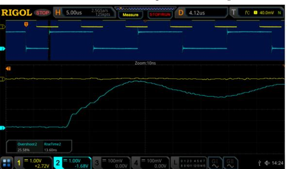
Figure 17: I2C data measurements with standard deviation using a RIGOL MSO5354 Digital Oscilloscope
