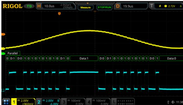
Figure 1: DAC output and input bit on a RIGOL MSO5354 Digital Oscilloscope
