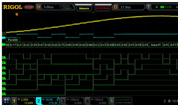
Figure 6: DAC output and 8 bit input bus triggered by a digital pattern on a RIGOL MSO5354 Digital Oscilloscope
