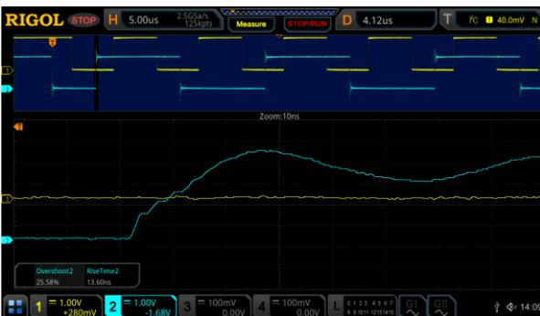
Figure 16: I2C zoom in on data risetime measurement using a RIGOL MSO5354 Digital Oscilloscope
