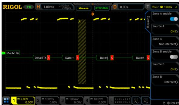
Figure 19: A zone trigger is added to exclude part of the RS232 signal.
