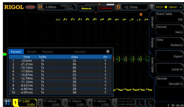
Figure 21: RS232 Event used to move around on the signal by using the Jump To soft key.
