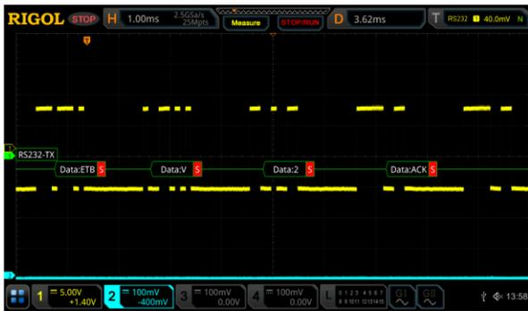
Figure 14: RS232 optional decoded data view settings using a RIGOL MSO5354 Digital Oscilloscope
