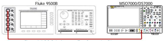
Figure 2-2 DC Gain Accuracy Test Connection Diagram
