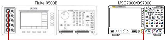
Figure 2-5 Timebase Accuracy Test Connection Diagram
