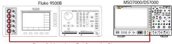
Figure 2-1 Impedance Test Connection Diagram
