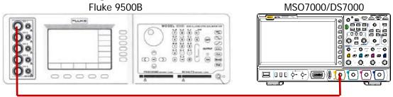
Figure 2-4 Bandwidth Limit Test Connection Diagram
