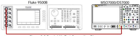
Figure 2-3 Bandwidth Test Connection Diagram
