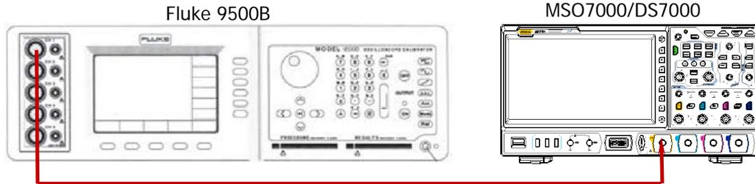
Figure 2-1 Impedance Test Connection Diagram
