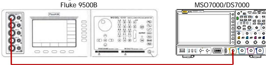
Figure 2-4 Bandwidth Limit Test Connection Diagram
