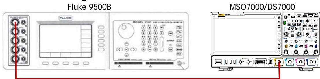
Figure 2-5 Timebase Accuracy Test Connection Diagram
