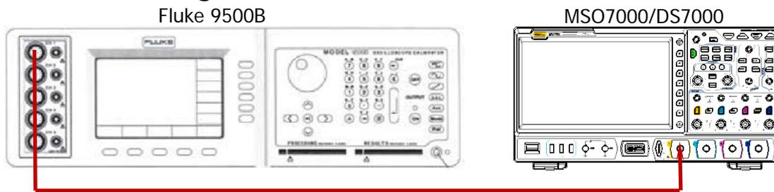
Figure 2-3 Bandwidth Test Connection Diagram
