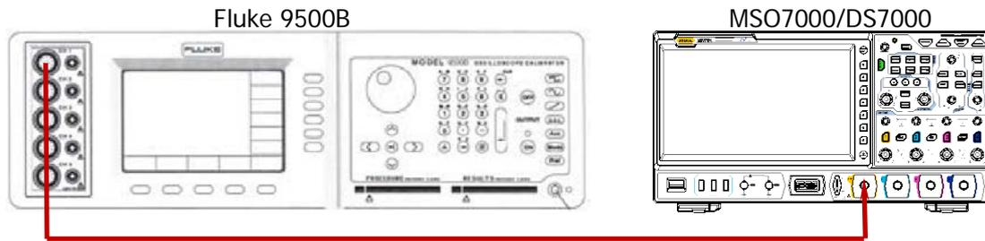
Figure 2-2 DC Gain Accuracy Test Connection Diagram
