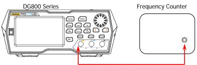
Figure 2-1 Connect DG800 and the Frequency Counter
