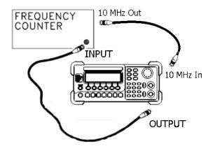
Figure 3-12 Frequency (External Timebase) Adjustment Connection
