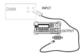
Figure 3-10 Output Impedance Adjustment Connection
