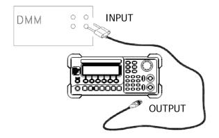
Figure 3-2 AC Amplitude Adjustment Connection
