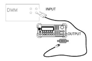
Figure 3-5 Output Impedance Adjustment Connection
