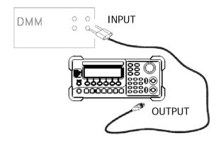
Figure 3-7 AC Amplitude Adjustment Connection
