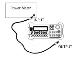
Figure 3-6 Output Flatness Adjustment Connection
