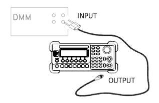
Figure 3-4 Low Frequency Flatness Adjustment Connection
