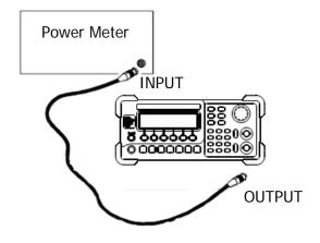
Figure 3-11 Output Flatness Adjustment Connection
