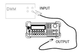
Figure 3-9 Low Frequency Flatness Adjustment Connection
