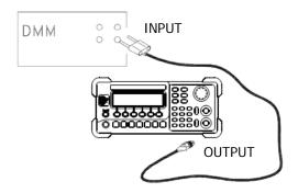
Figure 3-3 Offset DAC Connection
