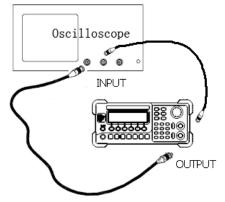
Figure 3-13 Phase Adjustment Connection
