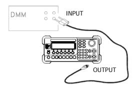
Figure 3-8 Offset DAC Connection
