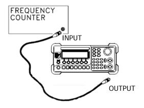
Figure 3-1 Frequency (Internal Timebase) Adjustment Connection
