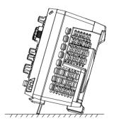
Figure 4 To Adjust the Supporting Legs
