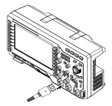
Figure 6 To Connect the Probe
