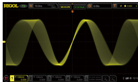
Changes of each frame of waveforms of the sweep signal can be clearly observed in high refresh mode.
