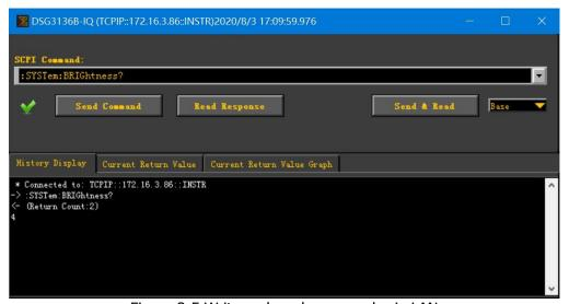
Figure 3-5 Write and read commands via LAN
