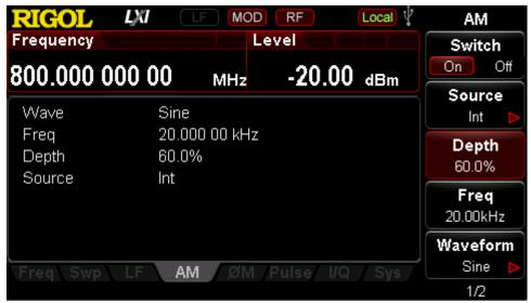
Figure 4-3 Parameter Setting Interface of RF Modulated Signal Output
