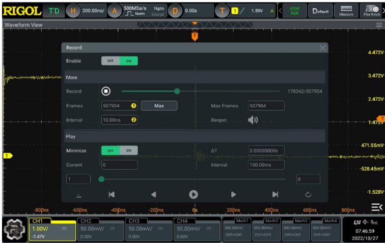
Figure 8: Record Mode Functions
