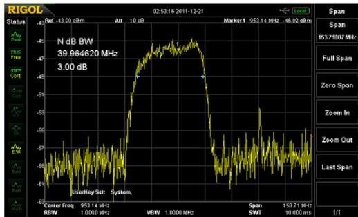
Some analyzers have a convenient Auto scale feature that can automatically configure the analyzer to display a full view of the area of interest on the trace.
