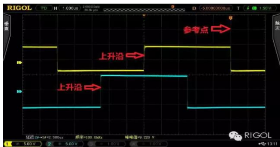
Figure 7. Testing C, D Signals Timing on Oscilloscope 2
