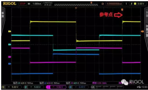
Figure 4. Four Lanes Time Delay Diagram
