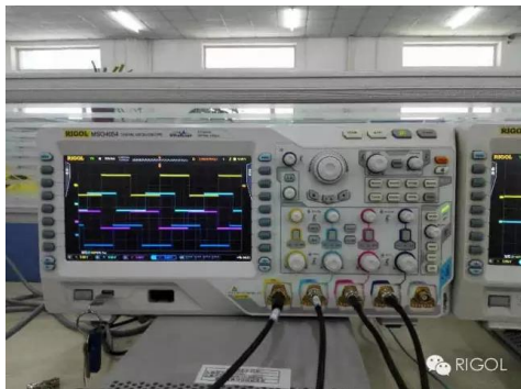
Figure 3. Testing for 4 Fixed Time-Delay Signal
