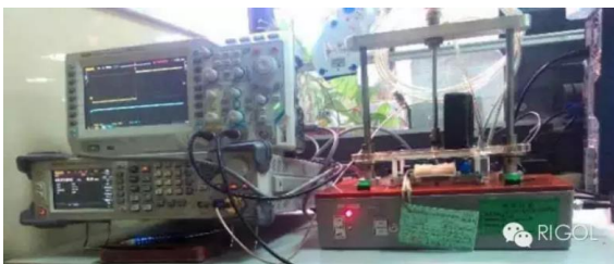
Figure 5 Wireless receiving end sensitivity and bit error rate testing
