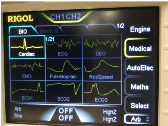
Figure 7 Arbitrary waveform generator built-in multiple arbitrary waveform
