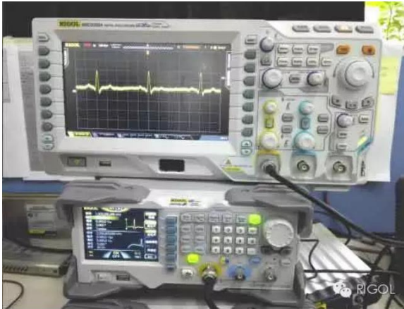
Figure 6 Arbitrary waveform generator generate low amplitude ECG signal
