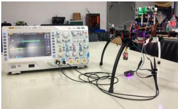
The flying controller debugging process by Oscilloscope
