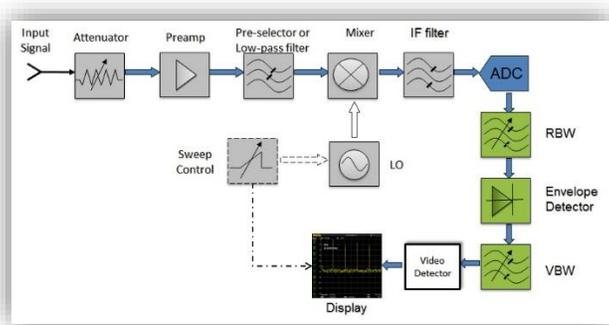
Spectrum analyzers based on swept super heterodyne designs are very popular. This is due, in part, to their low noise, ease of use, and ability to differentiate between signals that have very close frequencies.
