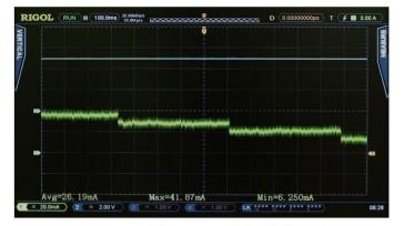
Figure 1: Current draw from program activating LEDs in succession
