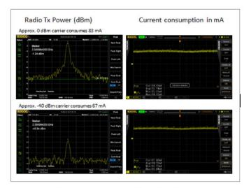
Figure 4: Current draw from Bluetooth Radio transmit test
