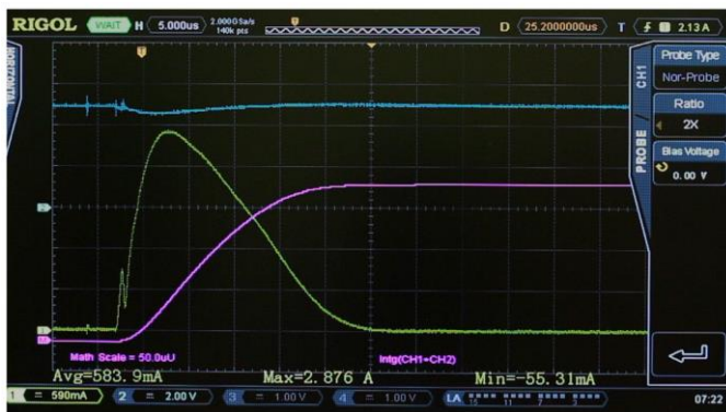
Figure 2: Hard Boot current spike and energy consumption of IoT platform
