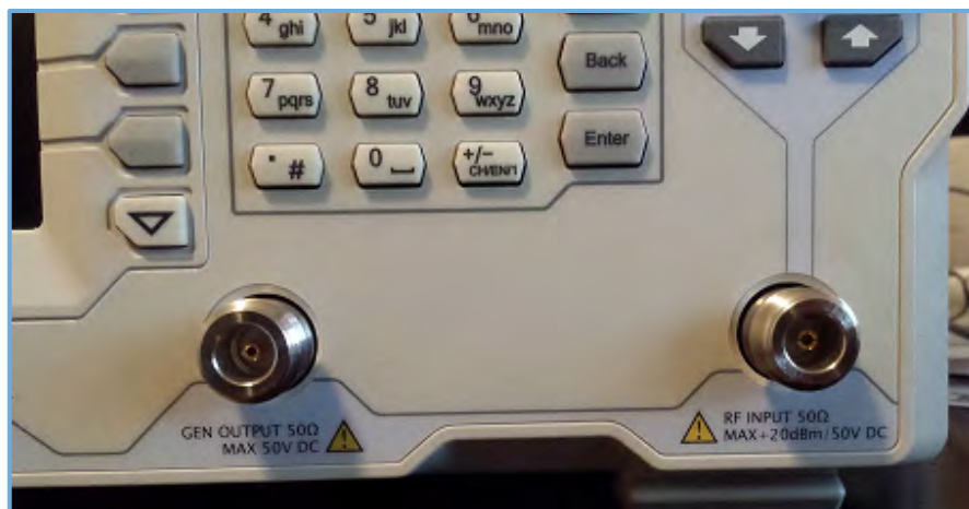
Figure 4-2: Front panel of a spectrum analyzer equipped with a tracking generator. This view shows connections to the RF output of the tracking generator and the RF input of the analyzer.
