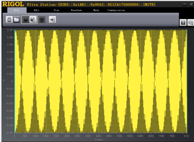
Figure 1: 400 cycles of Sine wave in an arbitrary waveform shown in Rigol Ultra Station Software
