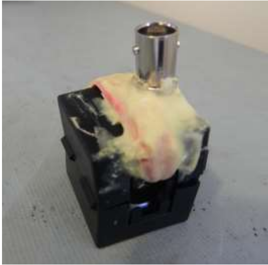
Figure 6: Homemade current probe.
