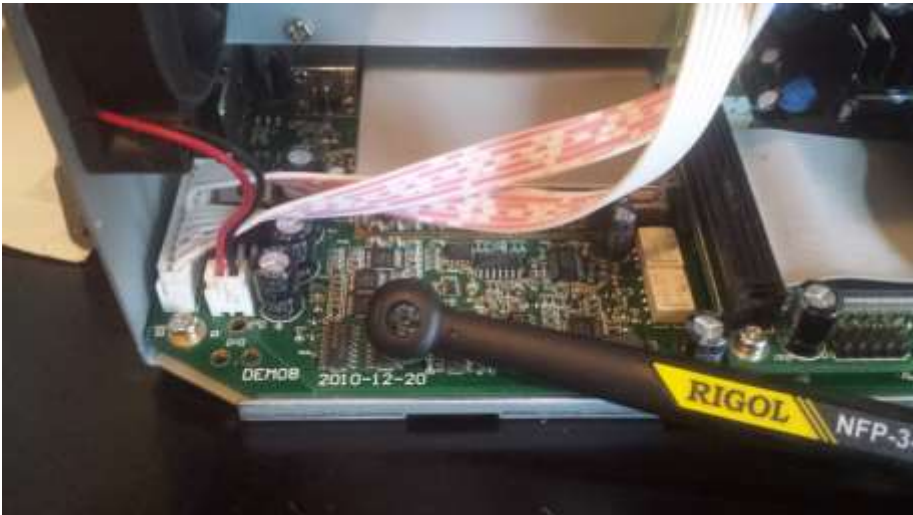
Figure 3: Using a near field probe on an unshielded Oscilloscope analog input circuit.
