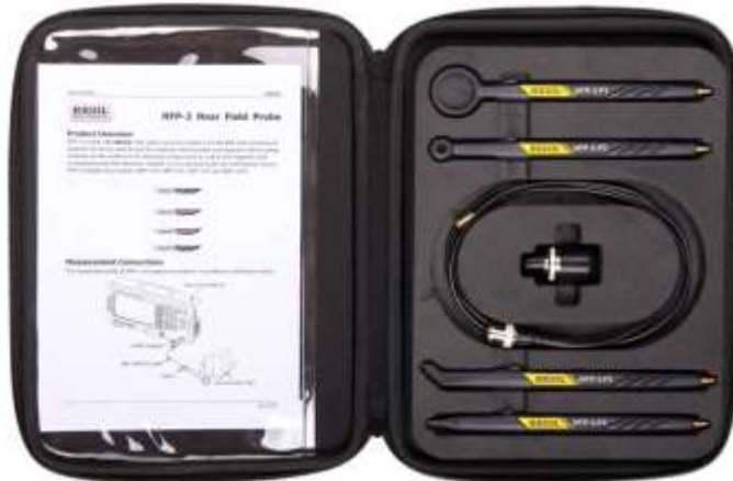
Figure 2: RIGOL’s NFP-3 set of Near Field Probes. These are all H field probes.
