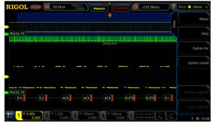
Figure 22: RS232 packet view using zoom mode on a RIGOL MSO5354 Digital Oscilloscope
