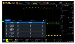
Figure 21: RS232 Event used to move around on the signal by using the Jump To soft key.
