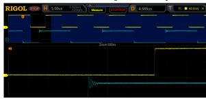
Figure 15: I2C clock and data min/max signal measurements using a RIGOL MSO5354 Digital Oscilloscope
