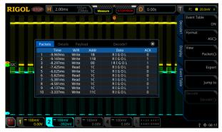
Figure 13: I2C clock and data event table view using a RIGOL MSO5354 Digital Oscilloscope
