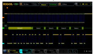
Figure 8: I2C clock and data with ground noise improved in a color graded display using a RIGOL MSO5354 Digital Oscilloscope your waveforms is vital to improved R&D efficiency and ultimately time to market.
