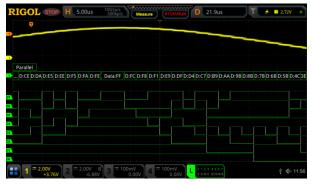
Figure 3: DAC output and 8 bit input bus with Hex decode on a RIGOL MSO5354 Digital Oscilloscope
