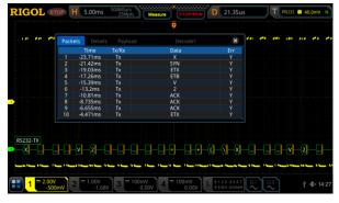
Figure 20: RS232 event table capture of multiple transmissions using a RIGOL MSO5354 Digital Oscilloscope
