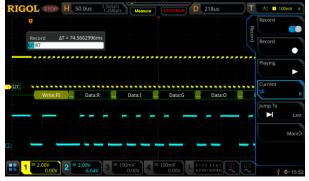
Figure 25: I2C transmission record mode in playback using a RIGOL MSO5354 Digital Oscilloscope
