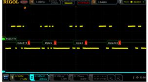
Figure 14: RS232 optional decoded data view settings using a RIGOL MSO5354 Digital Oscilloscope
