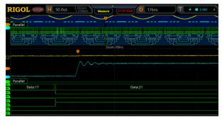
Figure 4: DAC output and 8 bit input bus zoomed in on a RIGOL MSO5354 Digital Oscilloscope
