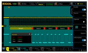
Figure 24: I2C with pass/fail analysis enabled using a RIGOL MSO5354 Digital Oscilloscope
