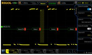
Figure 19: A zone trigger is added to exclude part of the RS232 signal.
