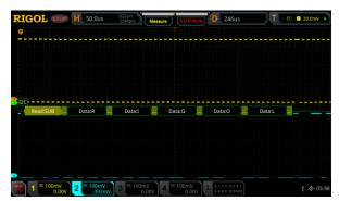
Figure 12: I2C clock and data using high resolution mode on a RIGOL MSO5354 Digital Oscilloscope
