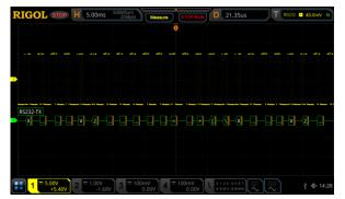
Figure 18: RS232 optimal decoded data view settings using a RIGOL MSO5354 Digital Oscilloscope
