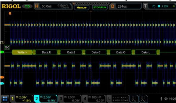
Figure 7: I2C clock and data with noise from poor grounding in a color graded display using a RIGOL MSO5354 Digital Oscilloscope
