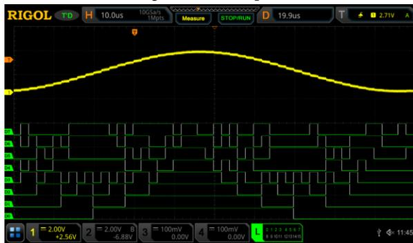
Figure 2: DAC output and 8 bit input bus on a RIGOL MSO5354 Digital Oscilloscope
