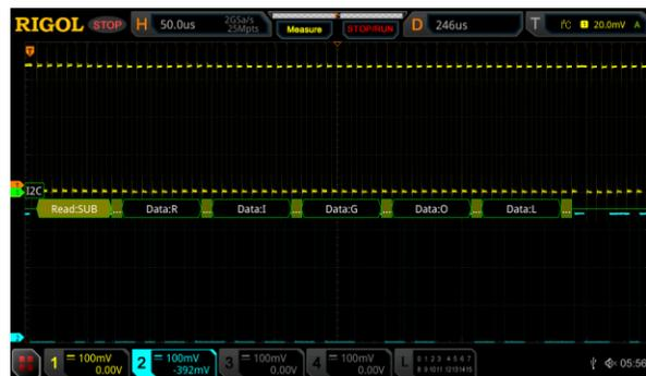
Figure 12: I2C clock and data using high resolution mode on a RIGOL MSO5354 Digital Oscilloscope
