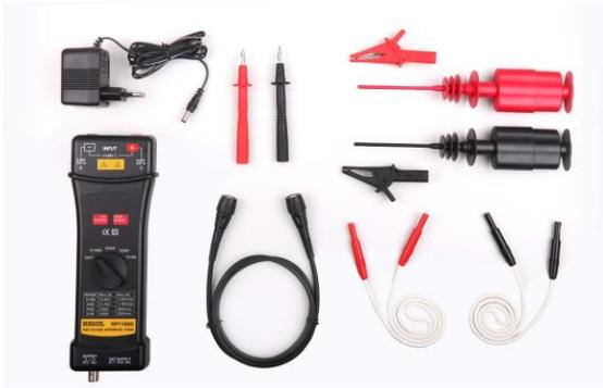
Figure 9: RP1100D 100 MHz Differential Probe
