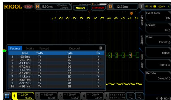
Figure 21: RS232 Event used to move around the signal by using the Jump To soft key.
