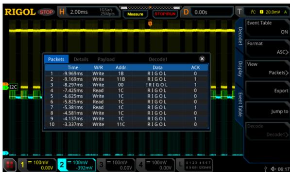
Figure 13: I2C clock and data event table view using a RIGOL MSO5354 Digital Oscilloscope
