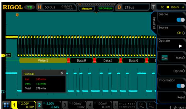
Figure 24: I2C with pass/fail analysis enabled using a RIGOL MSO5354 Digital Oscilloscope
