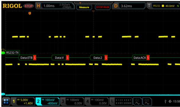
Figure 14: RS232 optional decoded data view settings using a RIGOL MSO5354 Digital Oscilloscope
