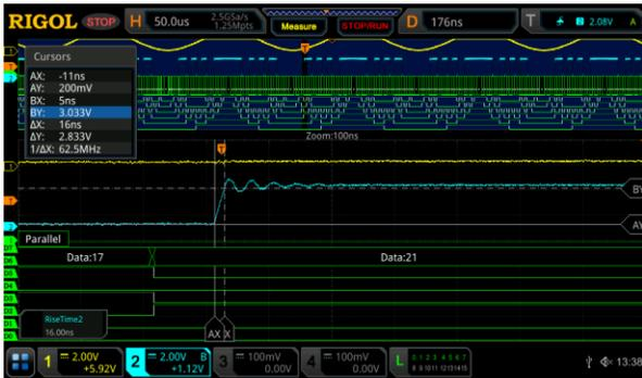
Figure 5: DAC output and 8 bit input bus zoomed in with cursors shown on a RIGOL MSO5354 Digital Oscilloscope
