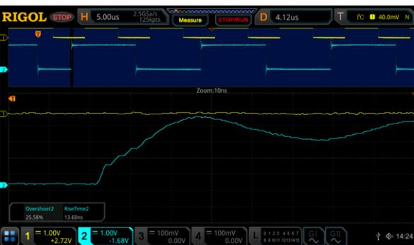
Figure 17: I2C data measurements with standard deviation using a RIGOL MSO5354 Digital Oscilloscope
