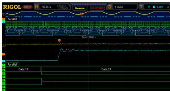
Figure 4: DAC output and 8 bit input bus zoomed in on a RIGOL MSO5354 Digital Oscilloscope
