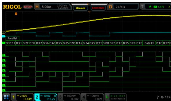
Figure 6: DAC output and 8 bit input bus triggered by a digital pattern on a RIGOL MSO5354 Digital Oscilloscope
