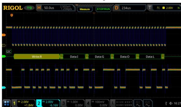
Figure 8: I2C clock and data with ground noise improved in a color graded display using a RIGOL MSO5354 Digital Oscilloscope
