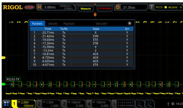
Figure 20: RS232 event table capture of multiple transmissions using a RIGOL MSO5354 Digital Oscilloscope
