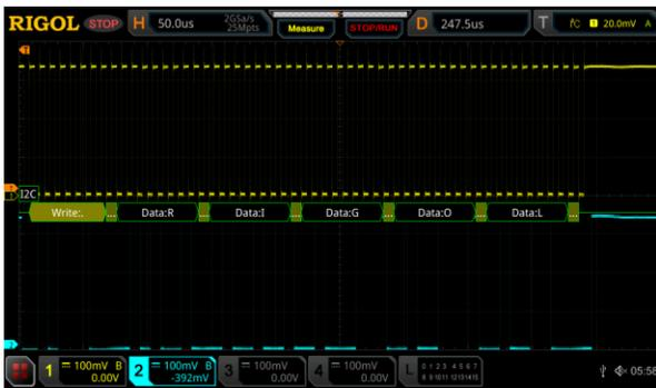
Figure 11: I2C clock data with reduced noise using bandwidth limit on a RIGOL MSO5354 Digital Oscilloscope
