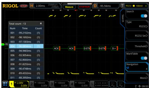
Figure 23: Using Search and Navigation feature to move around on the RS232 signal.
