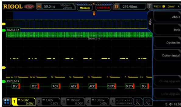
Figure 22: RS232 packet view using zoom mode on a RIGOL MSO5354 Digital Oscilloscope
