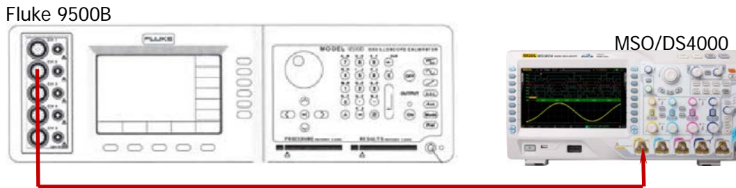
Figure 2-2 DC Gain Accuracy Test Connection Diagram
