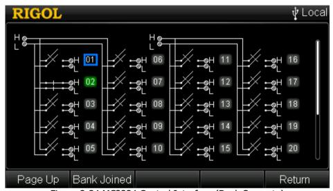
Figure 2-24 MC3324 Control Interface (Bank Separate)
