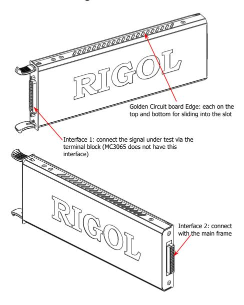
Figure 1-7 Outside view drawing of the module
