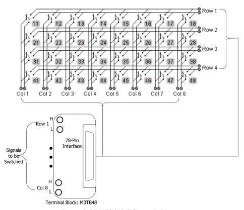
Figure 2-29 MC3648 Schematic Diagram
