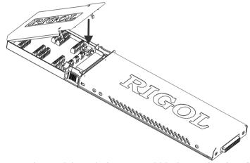
5. Insert the module with the terminal block into the slot of the mainframe.
