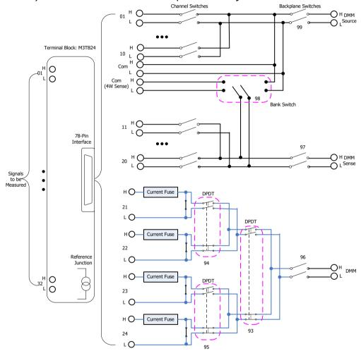
Figure 2-22 MC3324 Schematic Diagram
