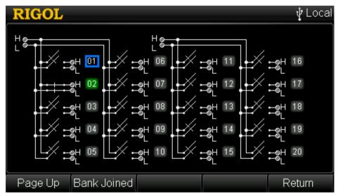
Figure 2-16 MC3120 Control Interface (Bank Separate)
