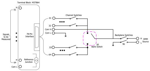
Figure 2-20 MC3164 Schematic Diagram
