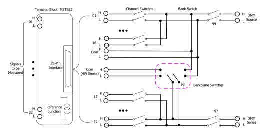
Figure 2-17 MC3132 Schematic Diagram
