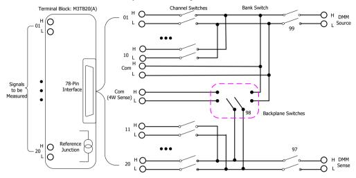
Figure 2-14 MC3120 Schematic Diagram
