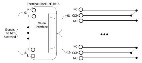
Figure 2-25 MC3416 Schematic Diagram
