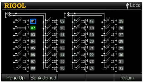
Figure 2-19 MC3132 Control Interface (Bank Separate)
