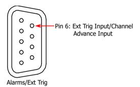
In external trigger mode, if the number of scans is set to "Infinite", after you press **Run/Stop** at the front panel, the instrument enters the wait-for-trigger state and then executes a scan each time an external trigger signal is received. Press and hold **Run/Stop** and the instrument will exit the wait-for-trigger state.
