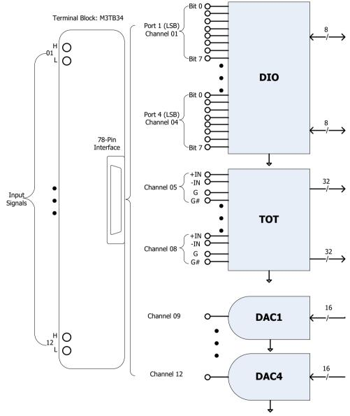
Figure 2-27 MC3534 Schematic Diagram
