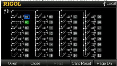
Figure 2-18 MC3132 Control Interface (Bank Joined)
