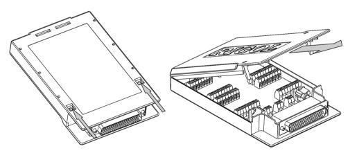
2. Connect the cables for connecting the signal under test according to the labels on the circuit board of the terminal block (for the connecting method, refer to Table 1-2). Pass the binding wires through the two groups of holes as pointed out by the arrows in the figure below to fix the cable connected. Pay attention
