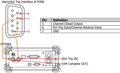
Figure 3-1 To Connect External DMM Schematic Diagram
