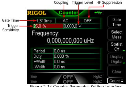
Figure 2-14 Counter Parameter Setting Interface
