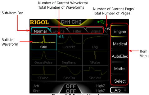
Figure 2-5 Built-in Waveform
