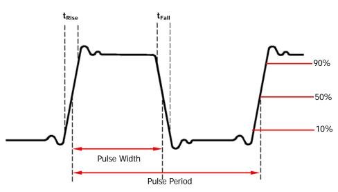
Leading/Trailing Edge Time  $\leq$  0.625  $\times$  Pulse Width
