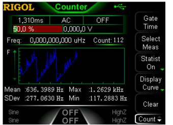
Figure 2-16 Statistic Results Interface (In "Curve" Display Mode)
