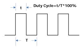
The setting range of duty cycle is limited by the "**Freq/Period**" setting. Please refer to "Signal Characteristics" in **"Specifications**". The default value is 50%.
