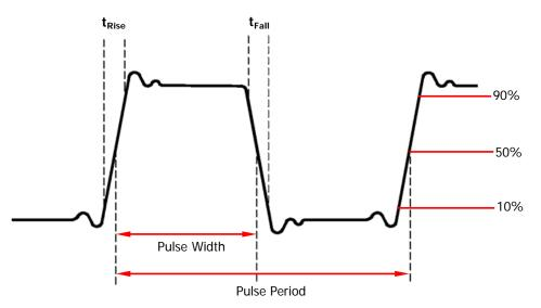
The setting range of pulse width is limited by the "Minimum Pulse Width" and the "Pulse Period" (for the ranges of "Minimum Pulse Width" and "Pulse Period", please refer to "Signal Characteristics" in "**Specifications**"). The range of pulse width is from 16ns to 999.999 982 118ks and the default value is 500µs.
