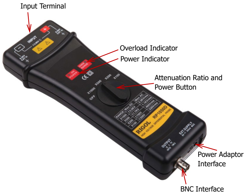
Figure 2 RP1050D High Voltage Differential Probe
