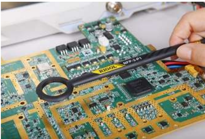
Figure 2: Near field E and H probes used to identify EMI sources
