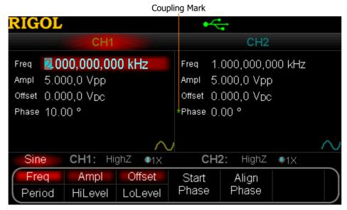
Figure 10-2 Channel Coupling
