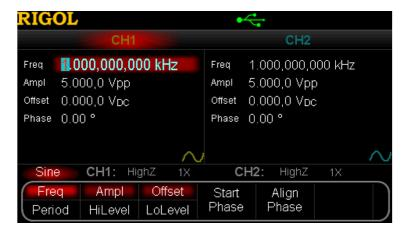
Figure 1-5 User Interface (Parameter Mode)
