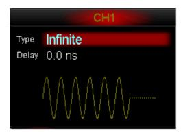
Infinite Burst could be triggered by "External" or "Manual" source. You can also set "**Start Phase**", "**Delay**", "**Trigger Input**" (external trigger) and "**Trigger Output**" (manual trigger).
