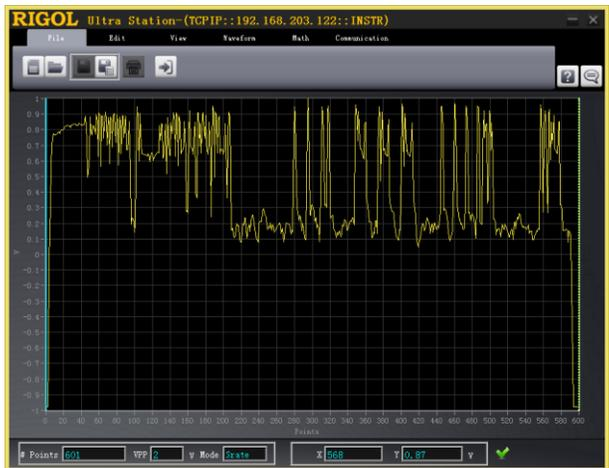
**Figure 8: UltraStation view of an arbitrary wave created from a spectrum analyzer capture**
