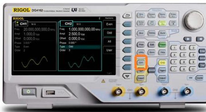
2. Press Freq/Period to toggle to Period. This shows the time duration of each period of the desired waveform.
