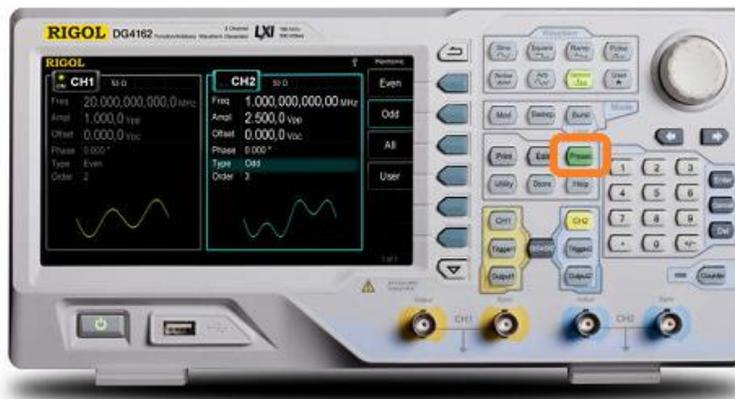
Alternately, you can set the PowerOn selection to Default by pressing Utility > System > PowerOn = Default and then power cycle the instrument.
