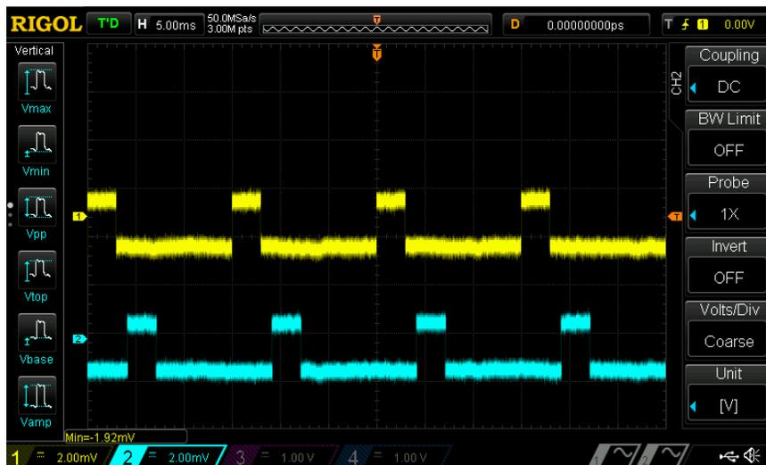
10. Align the phases by pressing CH1 and then press Align Phase
