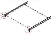
Secure the side beam fasteners to the cabinet by using four M6 screws and four M6 nuts.
