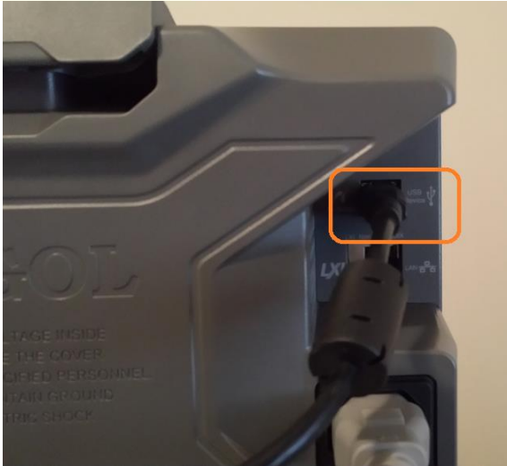
Figure 2: USB connection to DS1000Z series scope
