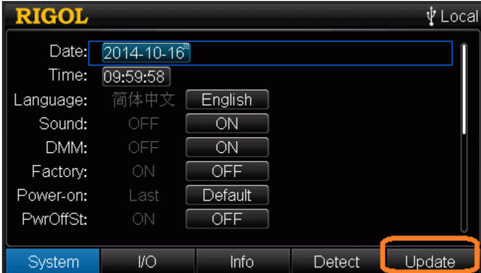
Figure 1: M300 Utility menu showing active UPDATE item present when a valid M300 firmware update file (*.UPD) is available on a USB memory stick on the front panel.
