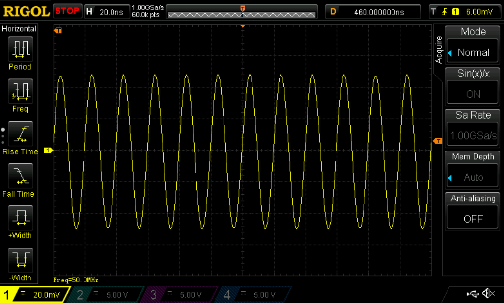
Figure 2 : 50MHz Carrier sine wave zoom.
