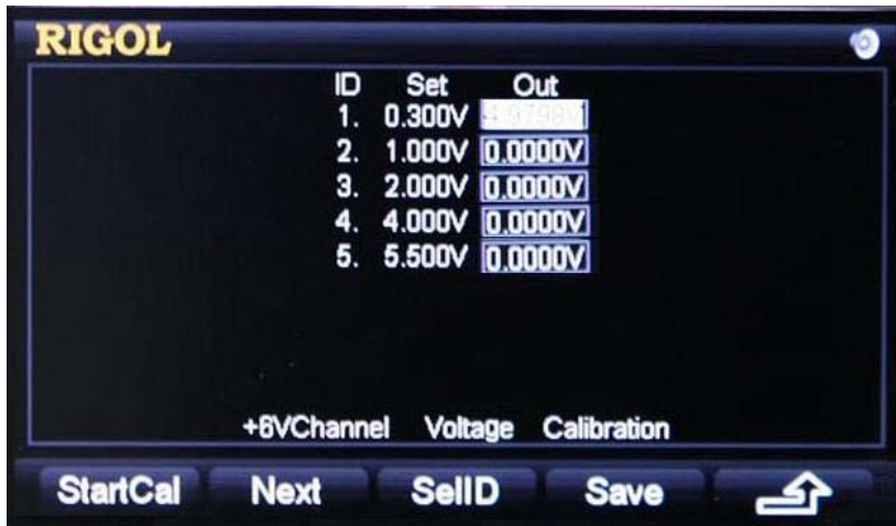
Figure 3-6 Voltage Calibration Interface
