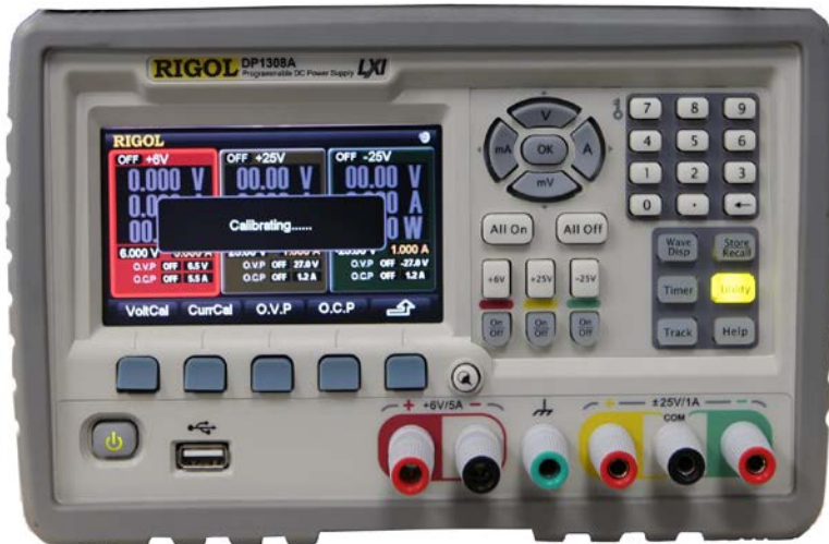
Figure 3-9 Overvoltage Protection Calibration
