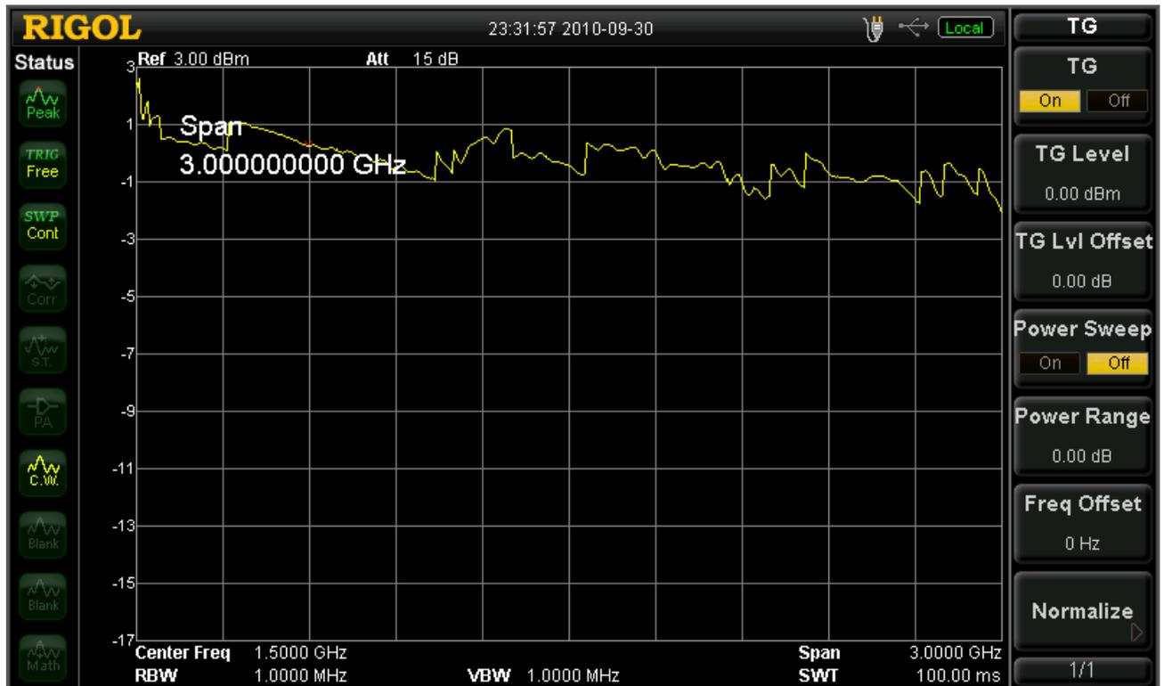
If the TG indicator at the top of the menu is set to off, then press the “TG” soft button to enable the Track Generator
