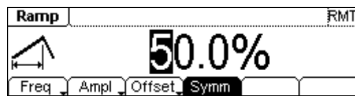
Figure 2-13 The Setting Interface of Ramp Signal
