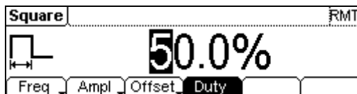
Figure 2-9 The Setting Interface of Square Signal
